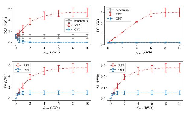
**Figure 5.** Mean and standard deviation values of the indicators D2P, PC, SV, and SL, see (15) to (18), over all days for different ESS capacities  $S_{\text{max}}$ .
