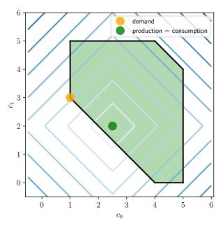
**Figure 3.** OPT in a simplified flexibility region (shaded region). The dark dot depicts the production signal to be tracked. The contour lines of the objective function are lines of constant L1-distance to the production signal. As the latter lies within the flexibility region, it coincides with the consumption returned by the OPT problem.
