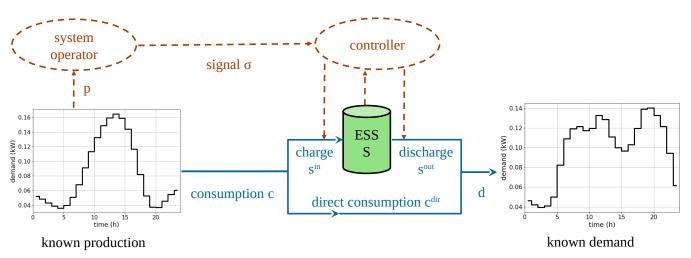
**Figure 1.** Energy system model: the power transfers between electric utility, ESS and household demand are indicated as solid lines. The dashed lines indicate signal communication (the signal which the electric utility sends to the household and the controller signals).
