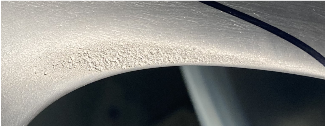
Figure 1.2: Erosion caused by cavitation on the backside of a bucket of a pelton wheel
