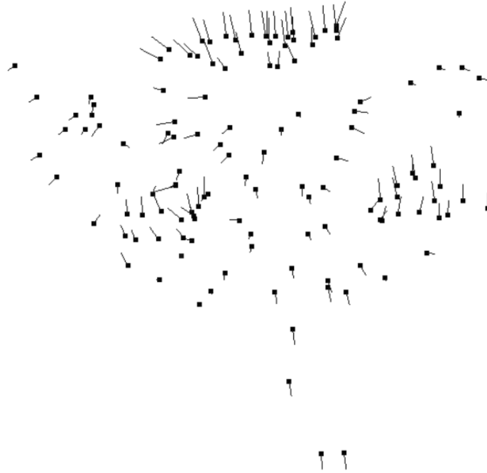
Figure 4.9: Target cloud with direction of normals depicted as lines. The cloud has 128 points.
