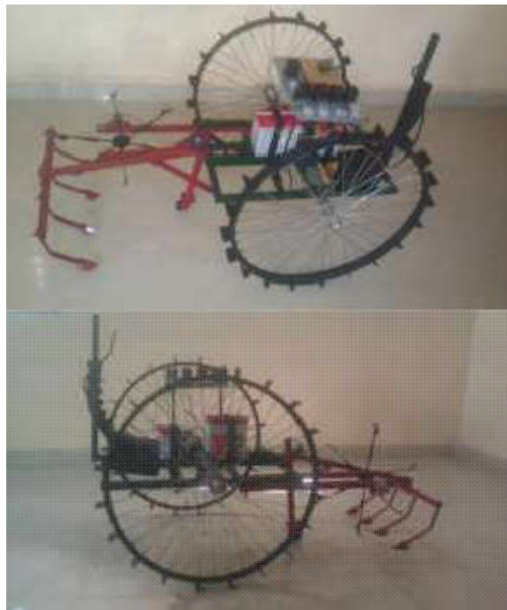
FIGURE 5. The mobile robot with a spraying system
